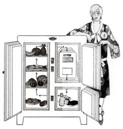
Arrows show how cold air and odors travel and how you should arrange food in your refrigerator. The coldest least odorous place, where milk and butter should be kept, is directly under the cooling unit. The warmest place, for strong-flavored foods, is the top shelf next to cooling unit
